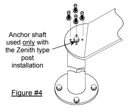
7) Lower the base cover over the post flange. Using the rubber mallet, tap the cover into place. Note: Tap gently to prevent denting the base cover.
