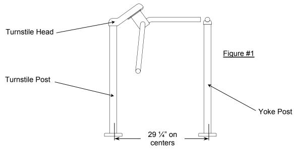
2) Anchor the posts per the vogue style or zenith style post installation instructions that are provided with this document. When using zenith style posts, completely tighten the outer four anchor bolts and <u>ONLY SEAT</u> the center anchor. Do not install the center anchor shaft at this time.
