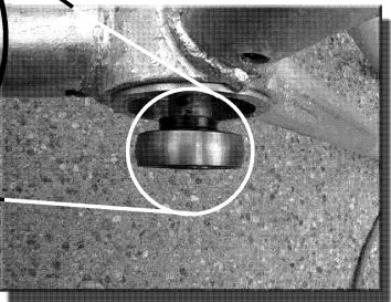
(Fig.9) Bottom bearing in correct position (flange "up")
