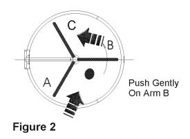
**WARNING:** Do not grab the Roto Section (A) and pull it in front of you. This will cause the Roto section to stop suddenly when the user is halfway through the turnstile.
