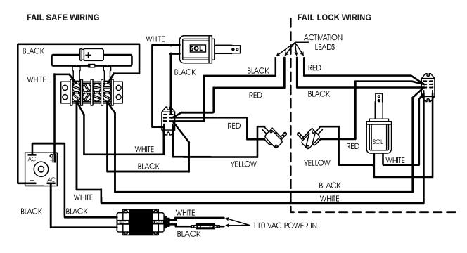
FAIL SAFE TIME DELAY RELAY WIRING
