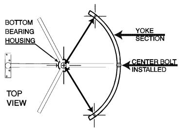
(Fig. 7) Measuring from center of bearing housing to outer yoke holes to equalize distance
