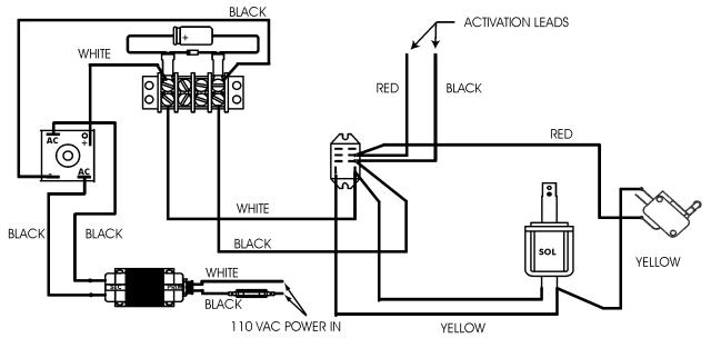
FAIL LOCK TIME DELAY RELAY WIRING
