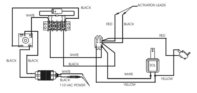
FAIL LOCK TIME DELAY RELAY WIRING
