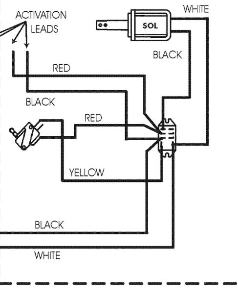
FAIL LOCK TIME DELAY RELAY WIRING
