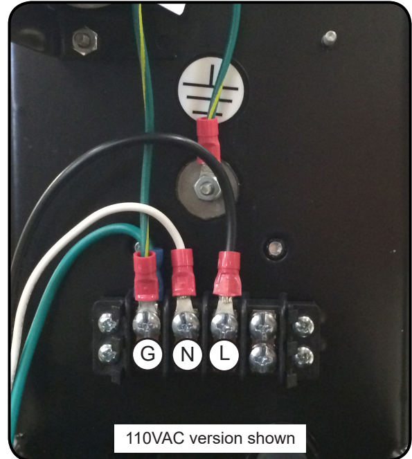
Fig. 17 Power Terminal Block
