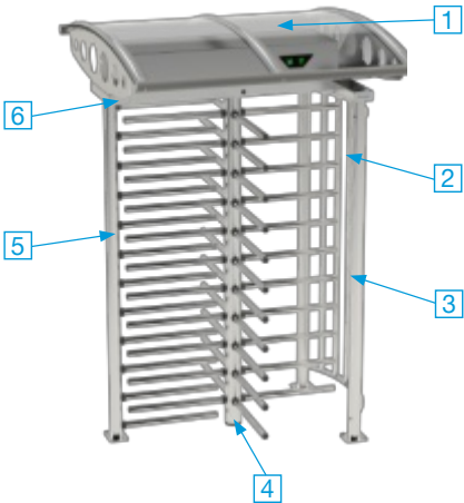
1. Canopy (option). 2. Passage way side frame. 3. Position for LED way Pictogram (option) and reader integration (option). 4. Rotor column with horizontal arms. 5. Stator bar frame. 6. Roof housing head mechanism and logic.
