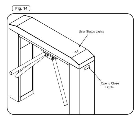
The EDM can also be equipped with Open / Close lights. The lights are installed on the upper "leg" of the cabinet and perform in the following manner [Fig. 14]:
