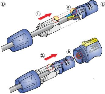
Slide the insert and the chuck (1) into the housing (2).
