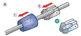
(A) Place the bushing (1) and the chuck (2) over the cable.
