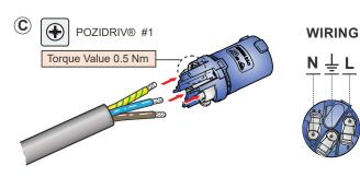
© Insert the wire into the terminals and fasten the clamping device with a POZIDRIV® #1, max. Torque 0.5 Nm (0.37 lb-ft).
