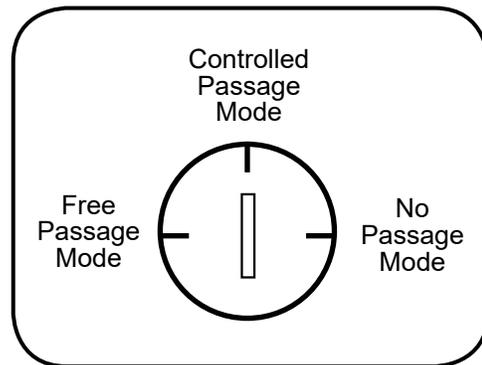
Turning the key to one of three positions overrides all existing settings, placing the turnstile in Controlled Passage mode, Free Passage mode or No Passage mode depending on the orientation of the key. Refer to the Passage Modes section on Page 15 for more information.
