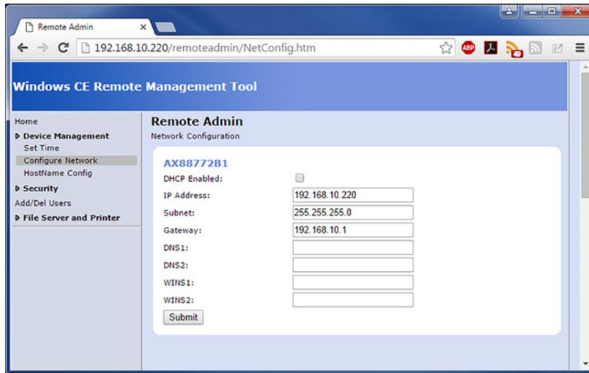
6. Wait for the Gateway to finish resetting. If the new IP address is on the same subnet as it was before, you will go back to the *Network Configuration* page. Otherwise, you will lose connection to the *Remote Admin* tool. Either outcome indicates the network configuration changed successfully.
