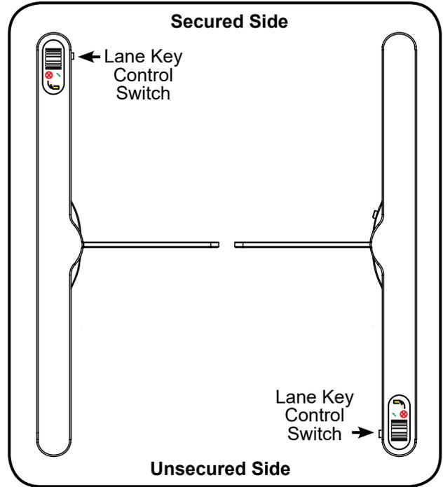
**Fig. 14** Lane Key Control Switch
