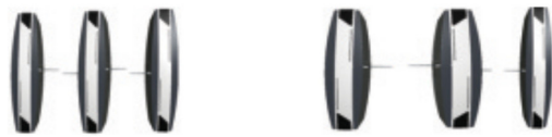
Two lane configuration comprising of 1N°L, 1N°C and 1N°R cabinets (left), and N°1 LW, 1N°CLW and 1N°R cabinet (right).
