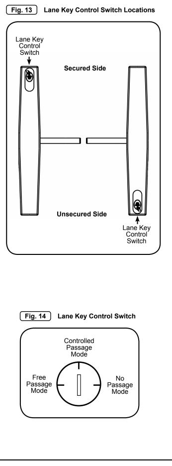
Turning the key to one of three positions overrides all existing settings, placing the turnstile in Controlled Passage mode, Free Passage mode or No Passage mode depending on the orientation of the key. Refer to the Passage Modes section on Page 15 for more information.
