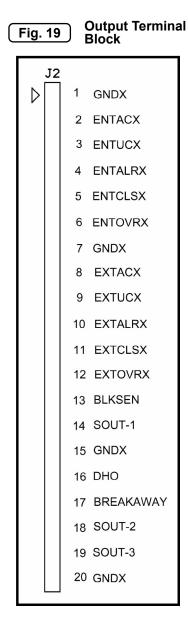
The following outputs are available to provide information on turnstile operational status and activity. All output contacts are 300ms in duration.
